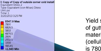
Yield strength of gutter material (cellular PVC) is 7800 psi
