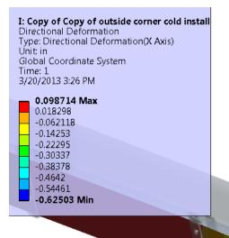
A gap of 0.625" between the gutter and fascia is necessary at the outside corners to accommodate the contraction of gutter into the fascia in this worst case condition. With the bracket being 0.125" thick, an additional 0.5" spacer must be used between the bracket and fascia.
